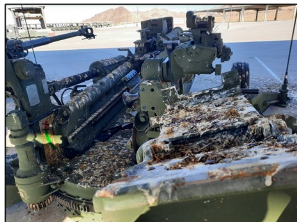
Photos 1 and 2. Raven Excreta Causing Damage at the at the 1 st Tanks Ramp at the Combat Center Desert in December 2021
